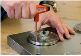
Uniformly loosen cylinder screws (2)
