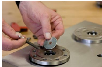
Insert installation tool (6)
