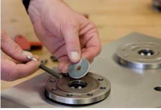
Remove installation tool (6)
