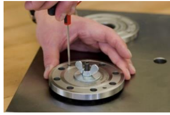
Screw in threaded pins (3) in order to be able to press down the clamping system
