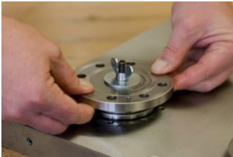
Uniform and tilt-free removal of the clamping module
