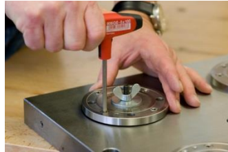
Uniform insertion of four opposing cylinder screws (2), up to flat contact.
